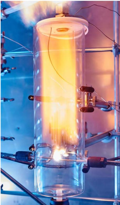
The determination of these characteristics is described in DIN EN 1839 and is performed by consilab according to the tube method (process T) (see figure on the left). The test mixture used is adjusted using mass flow controllers and consists of the test substance/fuel, air and, when determining the limiting oxygen concentration, also of additional inert gas (e.g. N<sub>2</sub>, water vapor).
