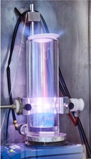
The characteristic value for assessing the ignition capability of an explosive atmosphere is the ignition energy. Ignition energy is the lowest amount of energy required to ignite an explosive atmosphere with a defined concentration.
