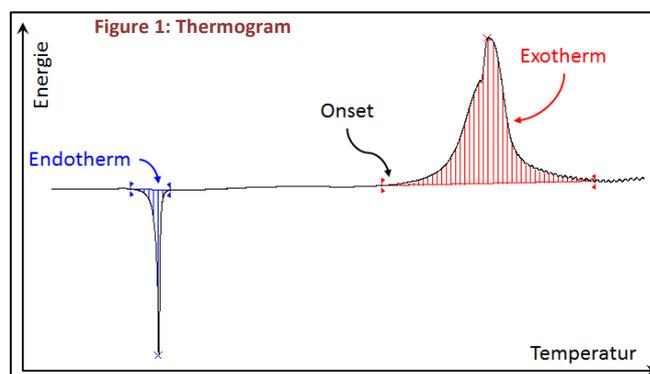
"onset temperature," a limit temperature " $T_{\text{exo}}$ " can be specified up to which a substance or mixture of substances is generally safe to handle. In accordance with the technical regulation for plant safety TRAS410, this limit temperature is set 100 K below the "onset temperature" of the first exothermic setting.
