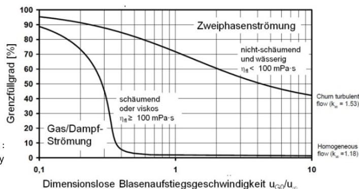
Fig. 2: Limit curves for determining the flow form as defined in ISO 4126-10
