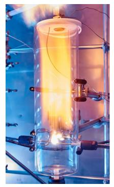
The test mixture is fed into a mixing chamber for homogenization. The fuel mixture is then fed into the cylinder-shaped explosion chamber and ignited with an ignition spark. Ignition occurs when a flame discharge from the ignition source is detected visually. To test the limiting oxygen concentration, an additional oxygen probe is installed at the exit of the explosion chamber, which allows oxygen to be continuously ascertained.
